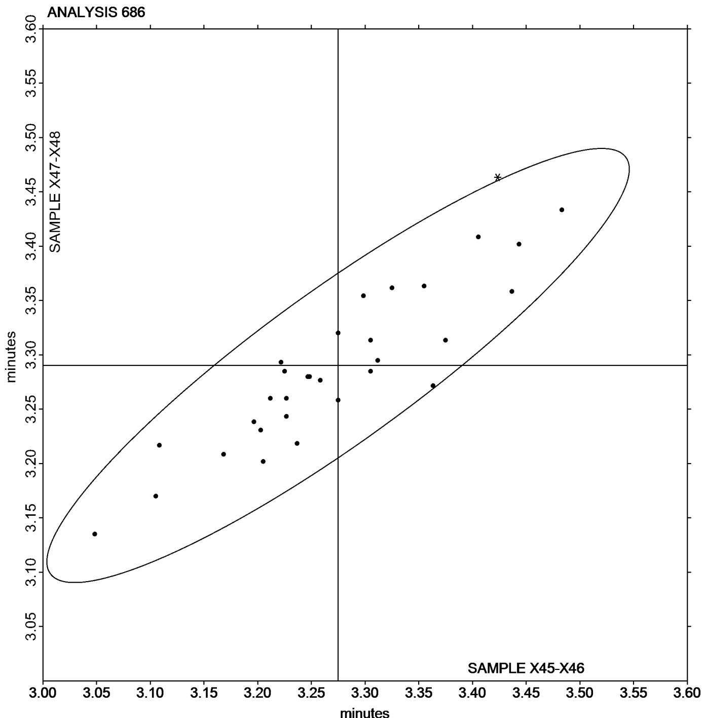
**Rubber Interlaboratory Testing Program****Analysis 687****MDR Vulcanization-Cure Time 90% (minutes)**
