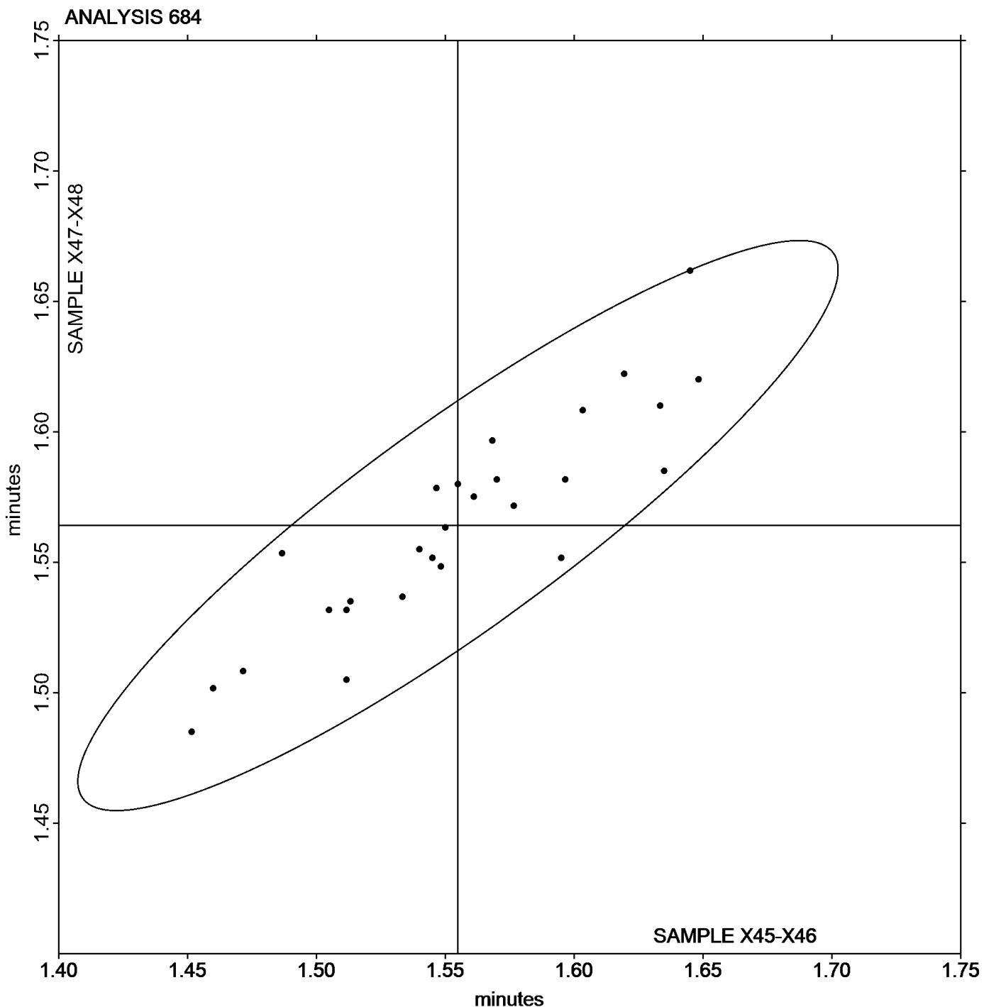
**Rubber Interlaboratory Testing Program****Analysis 685****MDR Vulcanization-Schorch Time, Ts1 (minutes)**
